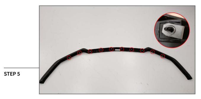
Remove the factory (10) metal speed clips, using a flat head screw driver, and transfer them to the new MMD chin spoiler.
