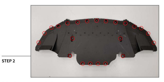
Using a 7mm socket and a flat head screw driver/trim panel removal tool, remove the splash shield.
