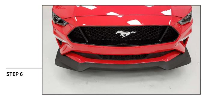
Install the MMD chin spoiler using the factory hardware, then reinstall the factory splash shield.
