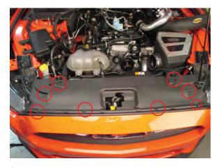
**Step 1** Remove the (8) clips securing the plastic radiator cover to the radiator support and remove it from the vehicle.
