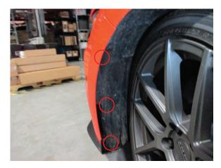
**Step 4** On each side of the bumper, remove the plastic clips holding the fender liner to the bumper.
