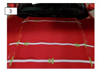
Gently place the hood scoop on the vehicle, center the hood scoop side to side and position the scoop far enough forward that there is clearance between the wiper arm and the back of the hood scoop. Tape the template to the hood as close to the edge of the scoop as possible. Remove hood scoop leaving template attached to the hood. Mark and carefully pre-drill the holes using a 1/8" drill bit. You will need to drill straight through the structural skins of the hood.
