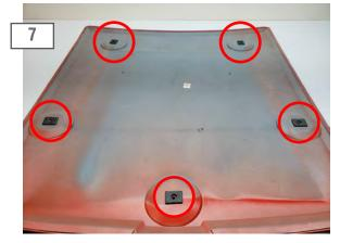
Peel the adhesive lining off the provided foam pads, and install them to the underside of the hood scoop around the mounting holes.
