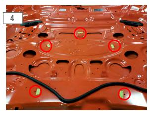
Once all holes have been drilled, enlarge the holes to 1/4". On the underhood side only (structural skin), enlarge the holes to 17/32" so that the hardware can pass through and sit flat on the underside of the hood skin.
