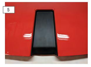
Using the alcohol prep pads, clean around the surface of the hood scoop that center insert will be applied. Peel back the red lining of the 3M tape, and carefully press on the center hood scoop insert.
