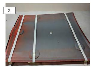
Align the (3) drill template sheets on the mounting locations of the hood scoop. Use painters tape to tape the edges of the hood scoop keeping the templates pulled tight.
