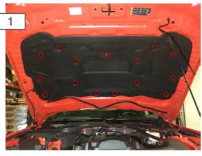
Begin by raising the hood to gain access to the under hood insulation. Remove the (15) push pins that hold the insulation liner to the hood using a trim panel removal tool.
