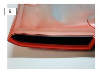
Using the alcohol prep pads, clean around the surface of the hood scoop that honeycomb insert will be applied. Peel back the red lining of the 3M tape, and carefully press on the honeycomb inserts to the hood scoop.
