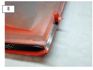
Clean hood with the supplied alcohol pads. Remove the red lining of the 3M tape all the way around the hood scoop.
