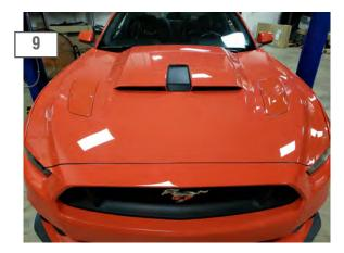
Loosely install the hood scoop with the provided screws and washers. Center the scoop side to side, then press fully around the hood scoop to ensure adhesion. Fully tighten the hardware. Reinstall the hood insulation liner. Installation is complete. \*\*Note: Do not over tighten the screws.
