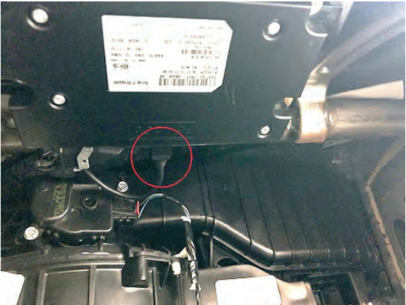
Step 10 (Sync Vehicles Only) Locate the USB connector on the Sync Module.
