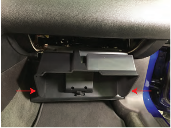
Step 9 (Sync Vehicles Only) Access the factory Sync module by lowering the glove box. Open the glove box and apply firm pressure to either side while gently pulling it down.
