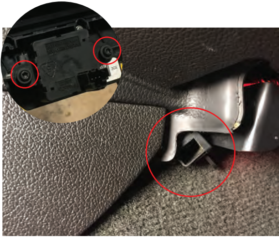
Step 7 (Dual Climate Control Only) To retain the "Auto" Fan speed control, remove the (2) T20 screws securing temperature sensor to the factory dash panel. Relocate the sensor to the passenger side foot well. There is space where the dash meets the carpet.
