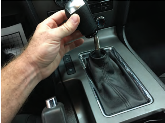
Step 1 Begin by removing the shift knob on manual transmission equipped vehicles or the shifter trim bezel on an automatic car.
