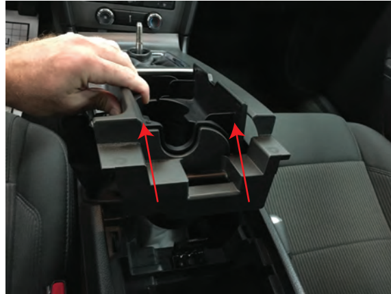
Step 2 Open the center console. Pull up on the back of the center console trim to remove.
