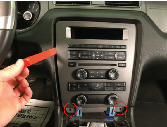
Step 4 Remove the (2) 8mm screws securing the dash trim panel to the vehicle. Then using a soft pry tool, gently pull the panel from the dash board. **Note: Steps 4-6 will be slightly different but very similar for vehicles with factory navigation.
