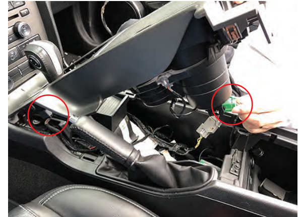
Step 3 Unplug all electrical connections. This includes the connection on the front left of the panel and the connection on the right side of the panel if applicable.
