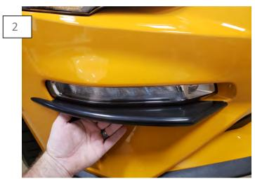
Before installing the bumper winglet, test fit the winglet to familiarize yourself with where it fits best.
