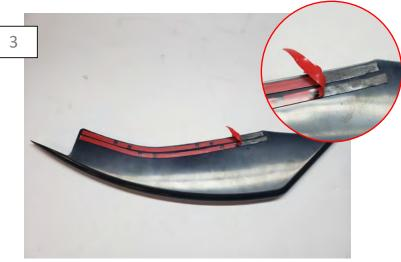
Apply the supplied 3M tape to the back side of the winglet. Test fit the part again before removing the tape backing.
