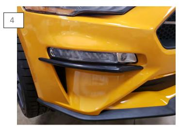
Remove the tape backing and Install the winglet to the under side of the light. Apply firm even pressure to the taped surface to ensure proper adhesion.
