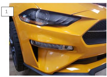
Begin by throughly cleaning the bumper with soap and water. Allow time for the bumper to dry. Using the supplied alcohol pad, clean under the light surface on both sides.
