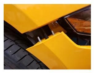
**Step 9:**Begin by removing the plastic bumper brace. Gently bend tabs as needed to remove support.
