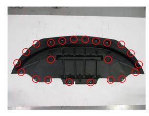
**Step 5:**On each side of the bumper, remove the plastic clips holding the fender liner to the bumper.
