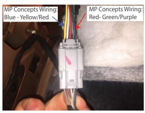
**Step 8**Using the supplied wire splice, tap the following:
