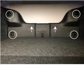
**Step 5**Remove the (4) twist on fasteners holding the trunk panel in place. Then apply slight upward pressure to remove the panel from trunk.
