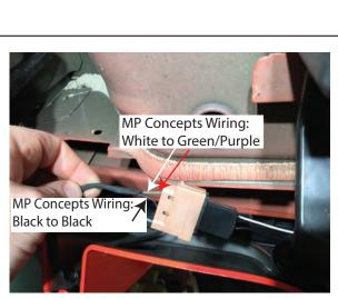
**Step 3**Connect the MP Concepts wiring to Factory wiring harness as follows.
