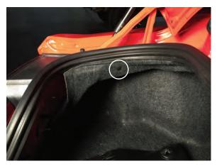
**Step 6**Using a panel removal tool or pliers, remove the plastic clip holding the trunk liner in place.
