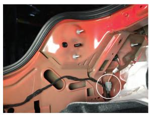
**Step 7**Fold back the trunk liner and locate the driver side tail light harness. Unclip the harness for easier access to the wiring harness.
