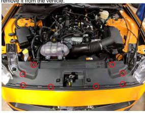
**Step 3:** Remove the (6) 8mm bolts, and (2) 6mm screws securing the bumper cover
