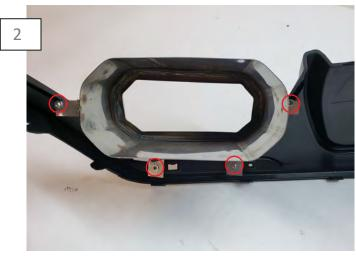
Secure the Quad Tips to the mounting locations using the provided screws. Do not fully tighten screws.
