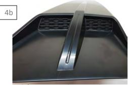
Apply firm pressure to the inserts making sure inserts adhere to the louver.
