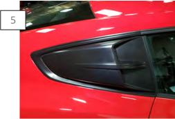
Fit the part before removing the tape backing. The louver should be aligned with the back corner and top edge first. Remove the tape backing, and apply firm pressure over all the tape surfaces.
