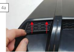
Install the inserts to the louvers by removing the tape backing and applying the inserts upward first then the bottom.
