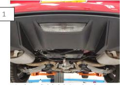
Using the supplied alcohol wipes, clean the rear diffuser fins and allow time to dry. Then use the promoter, and allow time to dry. \*\*Note: A clean surface is key to proper adhesion.
