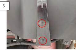
Once the holes are drilled, secure the fins fully using the supplied push clips.
