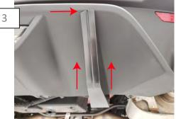
Install the diffuser fins by appling firm pressure on the fins and the factory rear diffuser. \*\*Note, begin at the front face of the fin first.
