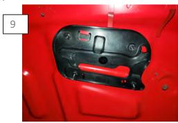
Remove the tape backing from step 7, and insert the hood vent into the hood. Secure hood vent using the factory (4) nuts.
