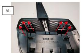
Insert the insert in an upward postion to meet with the upper edge, and then apply firm pressure to the taped areas.
