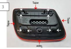
Remove the factory hood vent cover from the factory vent by releasing the plastic tabs and pulling away from the vent to release the tape adhesion.
