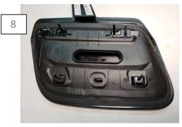
Install the factory hood vent cover from Step 3 onto the new hood vent by applying pressure till they click into place.
