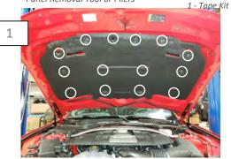
Remove the hood liner push pins and remove the liner to gain access to the factory hood vent mounting nuts.
