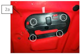
Remove the (4) 9mm nuts holding the factory vent in place. Then gently remove the factory vent from the hood.
