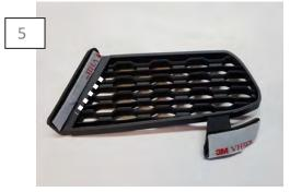
Install the supplied tape to the inserts area as shown above. \*\*Note: Some triming of the tape will be necessary.
