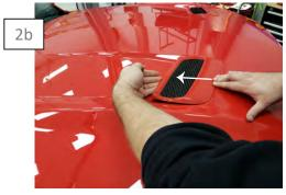
Carefully pull up on the back of the hood vent while gently pushing the front to release the factory clip securing the hood vent to the hood. Remove hood vent.
