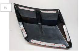
Once desired location is met, remove the tape backing from the scoop.
