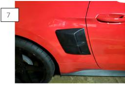
Apply firm pressure to the scoop over all the tape surfaces. Installation is now complete.
