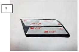
Apply the supplied tape to the (4) Inserts. The inserts will be labeled L-U for Left Upper, L-L for Left Lower, R-U for Right Upper, and R-L for Right Lower.
