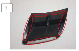
Wipe the tape edges on the scoop with the supplied alcohol wipes, allow time to dry. Then use the promoter, allow time to dry.
