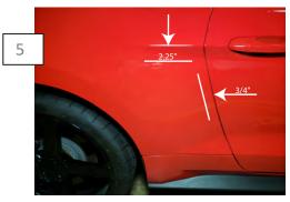
Fit the part before removing the tape backing. Messure roughly 2.25" inches from the body line down and roughly 3/4" inch from the door jam. Mark with painters tape.
