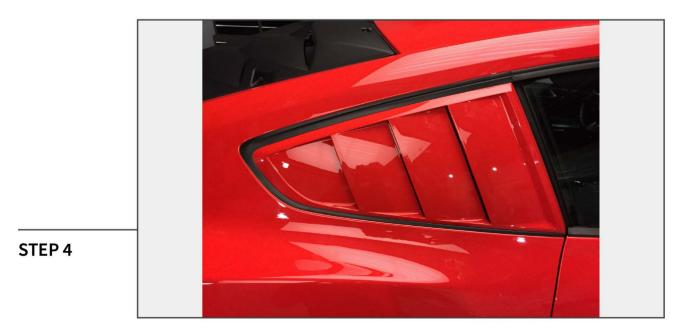
Before removing the tape's backing, test fit the louver on the window to familiarize yourself with how/where it fits the best. Ensure the window is clean before removing the tapes backing. Carefully install the louver onto the vehicle. Apply firm even pressure to the tape surfaces to ensure proper tape adhesion.
