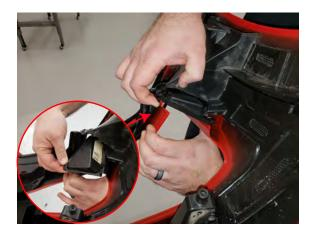
**Step 13:** Install the new bumper vents the same way the factory vents were removed.
