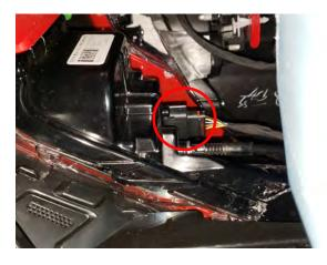
**Step 7:**On each side of the bumper, remove the plastic push clips holding the fender liner to the bumper.
