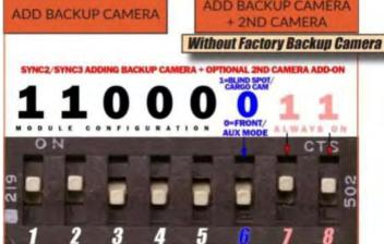
DIP Switches must be set before installation while the module is NOT connected to power for the module to work properly.
