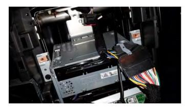
6. Remove (if plugged in) the 4-pin to 6-pin adaptor. It is not needed for installation.
