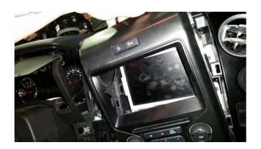
2. Remove the (4) 7mm bolts holding in the screen/display. Pull screen forward out of dash.
