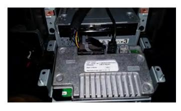
3. Remove the large plug to the left of the screen by lifting the handle like plug.
