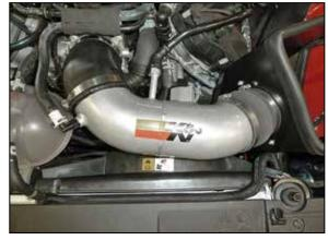
16. Install the intake tube into the coupler at the throttle body and onto the coupler at the filter adapter, adjust the tube for best fit and then secure the tube to the coupling hoses with the provided hose clamp. Connect the EVAP and crank case vent lines to the fittings installed into the K&N<sup>®</sup> intake tube.
