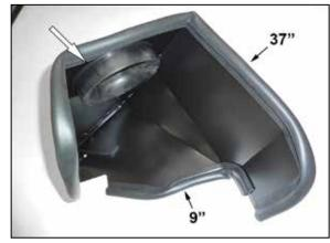
9. Install the provided edge trim onto the K&N<sup>®</sup> heat shield as shown. Install the air filter adapter into the heat shield and secure with the provided
