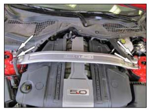
2. Remove the four nuts that secure the strut tower brace and then remove the strut tower brace from the vehicle.
