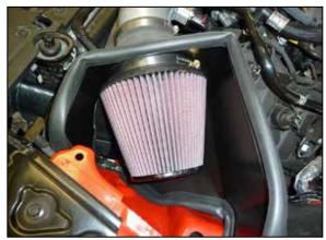
19. Install the K&N $^{\mbox{\tiny B}}$  air filter onto the filter adapter and secure with the provided hose clamp.
