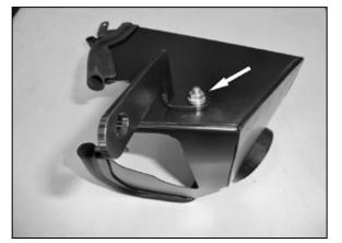
10. Install the provided mounting bracket (064357) onto the heat shield and secure with the provided hardware.
