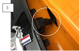
Unplug the reverse camera and remove the panel from the vehicle. Remove the (2) 5.5mm screws securing the camera to the panel. \*\*Note the orientation of the camera. If reinstalled backwards the camera will be inverted on the display. Reinstall the factory camera onto the MMD panel reusing the factory screws.
