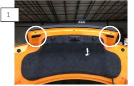
Using a panel removal tool, gently remove the caps covering the deck lid panel screws. Remove the (4) 7mm screws.
