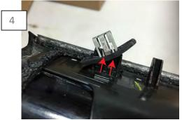
Remove the factory (4) push clips across the top of the decklid panel. Transfer these clips onto the MMD panel.
