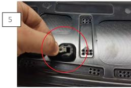
Remove the (4) factory screw clips across the bottom of the decklid panel. Transfer these clips onto the MMD panel.
