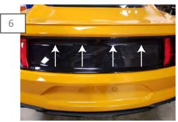
Plug in the camera and reinstall the decklid panel using the factory screws. Finish the install by reinstalling the factory screw covers.
