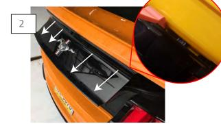
Using a panel removal tool, carefully separate the factory deck lid panel from the deck lid. It is clipped into the decklid along the top edge. \*\*Note: Do Not pry against the paint, decklid dents easily.
