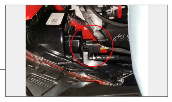
With the splash shield removed, disconnect the wiring harness from the turn signal/fog light housings.
