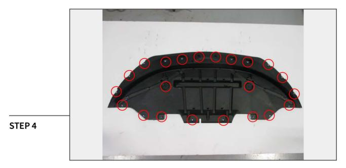
Remove the 7mm bolts & push clips attaching the splash shield to the bumper and undercarriage. There are two versions of the splash shield, both are attached similarly.
