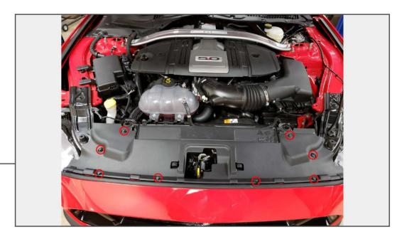
Jack the vehicle up and support the font end with jack stands. Using a trim panel removal tool, remove the (8) push clips securing the radiator cover and remove it from the vehicle.
