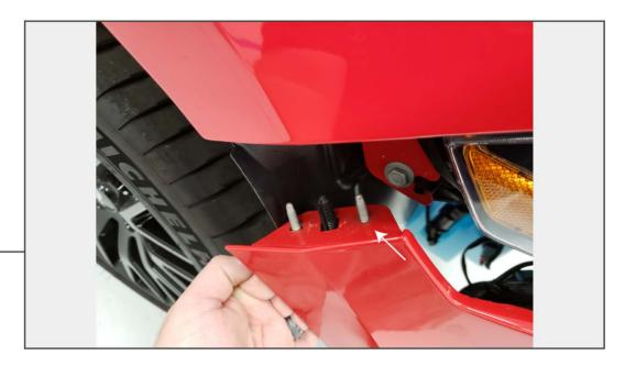
With the (2) 10mm nuts removed from the bumper bracket, you will still need to release the ribbed push rivet before the bumper will separate from the fenders. Take a long extension with a small socket and use it to push downward on the tip of the push rivet, this will push the rivet most of the way out. Gently pull down on the bumper to release the rivet the rest of the way. Remove bumper and set down on a non-abrasive surface where you can easily work.
