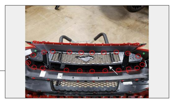
Using a large flat head screw driver, release the clips around the perimeter of the upper and lower grille. It's easiest if you start at the far left or right of the grille and work your way across.
