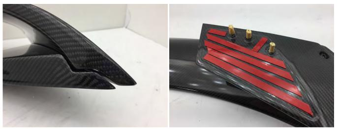
**Step 4**// Next, apply tape to the studs of the spoiler to avoid scratching the decklid paint. Center the spoiler on the back edge of the decklid and mark where you will need to drill the holes. Drill a 1/8" pilot hole. Finish drilling to a 5/16" hole. \*\*Note: The holes will need to be drilled slightly larger on the bottom side of the decklid to accommodate the flanged nut.
