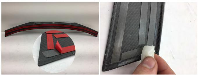
**Step 5**// Install the spoiler by centering it on the decklid. Apply firm even pressure on the spoiler to ensure proper adhesion.
