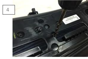
Remove the deck lid emblem by carefully removing the plastic weld from the back of the deck lid panel. Use an oversized drill bit and only remove enough material so that you can remove the emblem.
