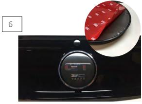
Test fit the emblem on the center of the decklid panel, then peel the 3M tape backing from the emblem. Center the emblem and apply firm even pressure to ensure proper adhesion to the decklid panel.
