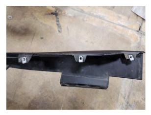
Step 9: Reinstall the diffuser to the bumper in the reverse order.
