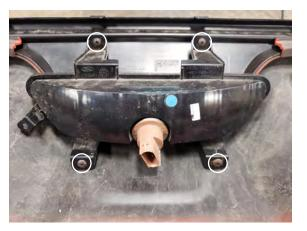
**Step 7:** Transfer the reflectors from the factory bumper to the new bumper. They are held on with a 10mm nut.
