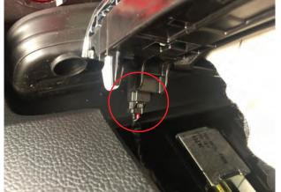
Step2\\ Apply firm pressure to the front edge of the shifter Remove the plug located at the left front of the bezel. bezel. Several clips secure it to the center console.
