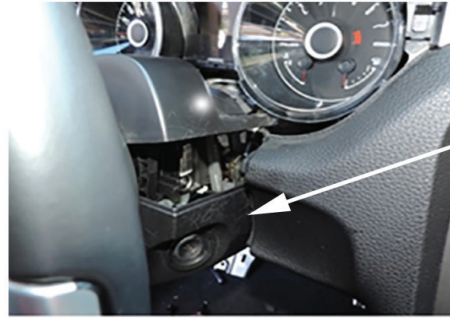
2. Lower Steering Wheel Shroud
