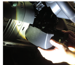
4. Pull Shroud down and forward
