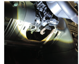
4. Pull Shroud down and forward
