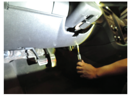
2. Remove 9/32" screw left side
