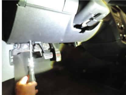
3. Remove 9/32" screw right side
