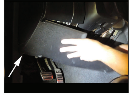
4. Pull down, slide out from corner
