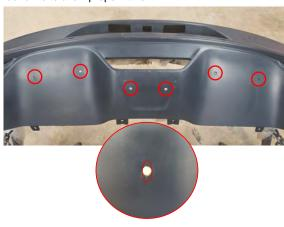
Step 15: Install the diffuser to the rear bumper using the (6) M8 nuts, and flat washers. \*\*CAUTION: DO NOT OVER TIGHTEN THE HARDWARE.
