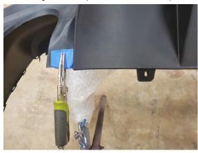
**Step 12:**Adjust the diffuser to make sure its perfectly centered on the rear bumper.
