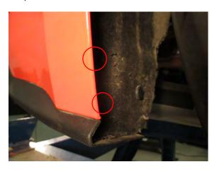
**Step 3:** Fold the fender liner out of the way to access the (3) bumper cover bracket bolts.
