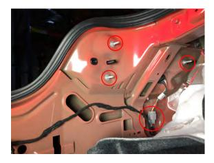
**Step 7:**Pull the bumper away from the vehicle on both sides.
