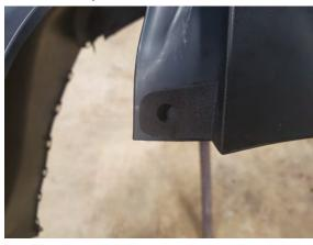
**Step 17:**Secure the side tabs to the bumper using the supplied 1/4" plastic push clips.
