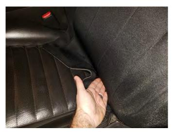
**Step 4\\**Secure the upper portion of the seat cover by tucking the velcro sleeve in-between the upper and lower parts of the seat and velcro in place.
