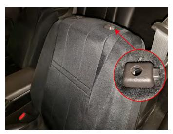
**Step 3\\**With the headrest still removed, pull over the upper seat cover portion. Tuck the seat cover under and around the headrest guides.
