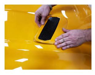
**Step 3:**Using a 10mm socket and ratchet, install the (4) studs to the MP Concepts hood vent.
