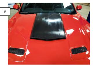
Test fit the hood scoop. Then remove the hood scoop to remove the double side tape backing. Align the scoop. Using the supplied washers and nuts, secure the hood scoop to the vehicle. Once secured, apply firm even pressure to the taped locations to ensure proper adhesion. Installation is now complete.
