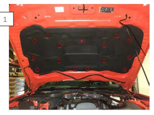
Begin by raising the hood to gain access to the under hood insulation. Remove the (15) push pins that hold the insulation liner to the hood.
