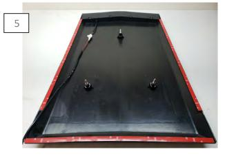
Optional Lighting- Connect the scoop lighting to the control box. \*\*Note: Secure the light wiring to the under side of the hood scoop using a quality adhesive backed tape. Then mount the control box in the engine bay using a quality adhesive backed tape.
