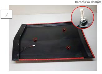
Wash the hood with soap and water. Allow the panel time to dry. Apply the supplied 3M double sided tape to the ledge areas. Then insert the (3) studs and nuts into the hood scoop.
