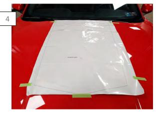
Align template across the back edge of the hood and centered between the cowl ridges. Tape the template in place so that it doesn't move while drilling. Before drilling, raise the hood slightly to avoid drilling through any engine components. In most of the locations you will be drilling through the outer and inner hood. Pre-drill the (3) holes using a 1/8" drill bit. Finish drilling the holes to 9/32". \*\*Note: Apply touch up paint to any bare metal to prevent oxidation.
