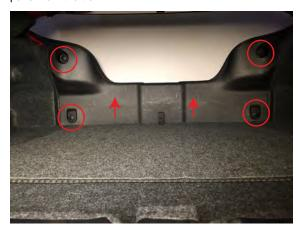
**Step 2:** Using a trim panel removal tool, remove the plastic push clip holding the trunk liner in place.
