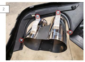
Secure the Quad Tips to the mounting locations using the provided screws & washers. Do not fully tighten screws.
