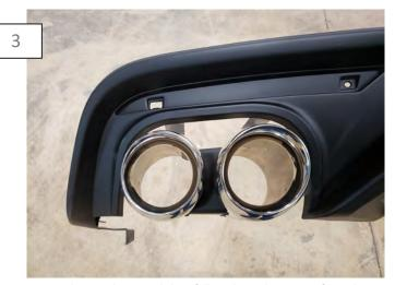
Center the Quad Tips and then fully tighten the screws from the previous step. \*\*Note: Do not over tighten the screws. Doing so can pull the threads out of the bosses.
