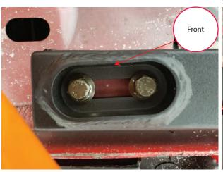
the (2) M10x1.5x25mm bolts to secure the rail to the body.
