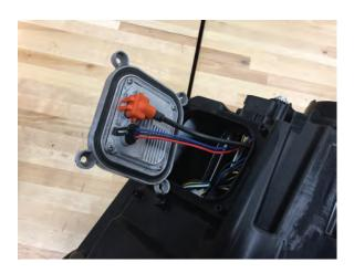
**Step 19**Plug in the connectors to the factory ballast. Install the ballast to the new headlight using the factory (4) T20 torx screws from Step 9.
