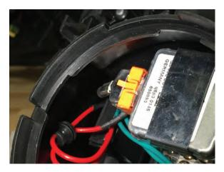
**Step 17** Insert the factory wiring harness from Step 11 through the new headlight, and plug in the connector to the headlight bulb.
