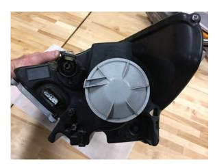
**Step 10**Carefully twist the factory headlight bulb cover counter-clockwise. Remove cover.
