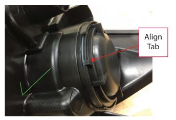
**Step 18b**Reinstall the headlight bulb cover by carefully twisting it clockwise. \*\*Note: Be sure to align the cover properly with the headlight housing. This deminstration shows it correctly installed.
