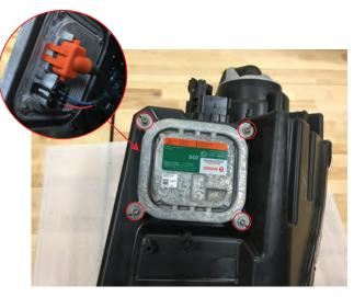
**Step 9**Remove the (4) T20 torx bit screws from the factory ballast. Then unplug both connections. \*\*Note: Hardware and cover will be reused in a later step.
