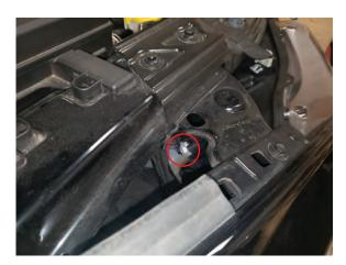
**Step 21**Using a Phillips or Allen key, use the attached adjustment screw to adjust the headlight to the factory specifications which can be found in the owners manual.
