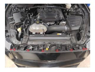
**Step 2**Remove the (6) 8mm and (2) 5.5mm bolts securing the bumper cover to the radiator support.
