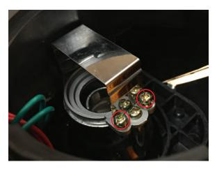
**Step 14**Using a phillips head screw driver, remove the (2) outer screws and carefully bend back the headlight bulb retailing bracket.
