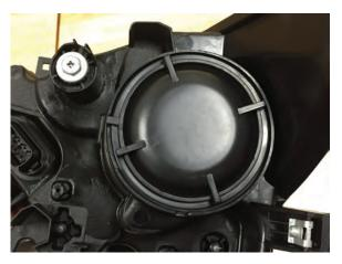
**Step 13**Carefully twist the headlight bulb cover counter-clockwise from the new headlight. Remove cover.
