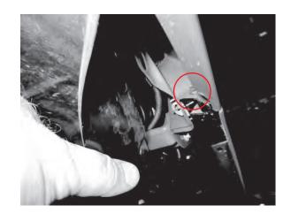
**Step 5**Fold back the fender liner so that you can access the one bolt that holds the bumper to the fender. Once removed, firmly pull the sides of the bumper away from the fender.
