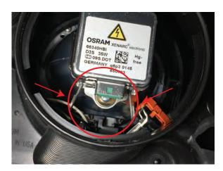
**Step 11**Unplug the connector to the headlight bulb. Then using a small flat head screw driver, remove the bulb retaining clip. Remove the bulb from the socket.
