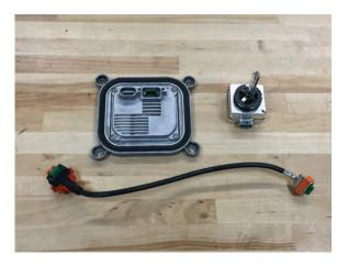
**Step 12**\*\*Note: The factory wiring harness, HID headlight bulb, and ballast will be transfered to the new headlight.
