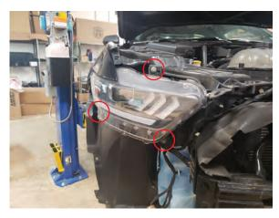
**Step 7**Remove the factory 10mm and 13mm hardware from the vehicle. Then remove the headlight.
