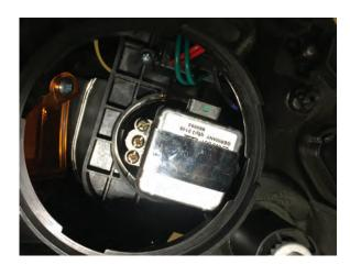
**Step 16**Reinstall the headlight bulb retaining bracket and the (2) screws to secure the bulb to the socket.
