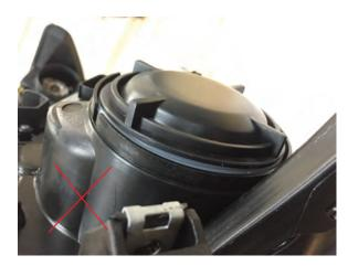
**Step 18a**Reinstall the headlight bulb cover by carefully twisting it clockwise. \*\*Note: Be sure to align the cover properly with the headlight housing. This deminstration shows it incorrectly installed.
