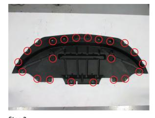
**Step 3**Support the front of the car so you can access the bumper splash shield. \*\*Note there are two versions of the splash shield. Both are attached to similar locations.
