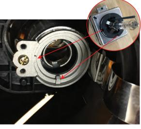
**Step 15**With the headlight retaining bracket bent back, install the factory HID bulb into the new headlight. Be sure to align the tabs from the bulb with the tabs of the headlight socket.
