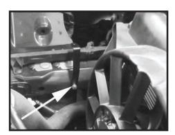
Step 6 Using the supplied hardware, install the "L" bracket onto the frame using the hole that is threaded. This is located towards the front of frame on the driver's side.
