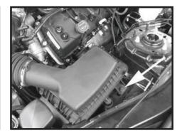
Step 4 Remove the factory air box and tube assembly by removing the 10mm bolt and lifting it out.
