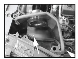
Step 7 Install the heat shield and secure it using the supplied hardware. Fully tighten all mounting hardware.
