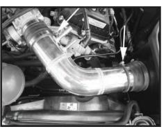
Step 10 Install the intake tube. Once in the desired location and everything fits in place, tighten the clamps.
