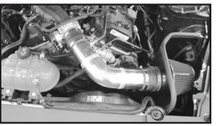
Step 12 Make sure that all clamps and hardware are fully tightened. Reconnect the battery cable, start the vehicle and let it warm up. Shut off and inspect the installation once more for any loose clamps, wires, or hardware. Test drive & enjoy! Your installation is now complete. Periodically check all clamps and brackets.
