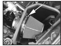
Step 9 Install the filter and securely fasten to the velocity stack adaptor.
