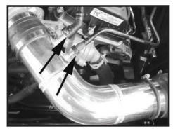
Step 11 Reconnect the factory vent lines to the intake tube.
