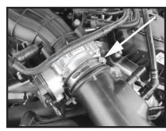
Step 3 Loosen the hose clamp at the throttle body.
