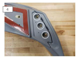
Attach the side mounts to the spoiler using (3) philips head screws, and flat washers.
