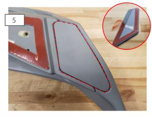
Using the supplied alcohol pads, clean around the surface of the spoiler bracket that tape will be applied. Allow time to dry. Peel back the red lining of the 3m tape, and carefully place the side bracket cover onto the side brackets. Press around the areas being applied with tape to secure.
