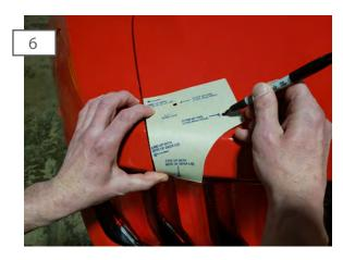
Using the supplied template, align the edge of the template with the edge of the trunk lid. Mark the holes that will be drilled.
