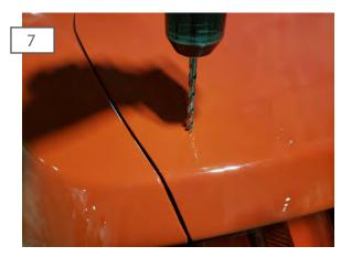
Using a 1/4" drill bit and drill, carefully drill the center of the template holes. \*\*Note: Use touch up paint to cover any exposed metal to prevent rusting.
