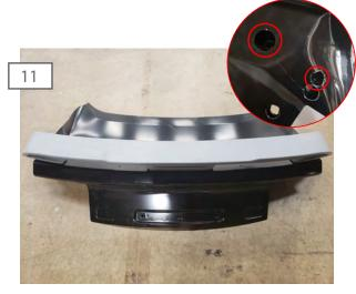
With a helper, start each of the (2) screws, (2) washers and nuts to hold the spoiler in place. Once the spoiler is loosely mounted, peel the tape backing off. Apply firm even pressure to tapped surfaced to ensure proper adhesion. Then fully tighten the hardware. Reinstall the interior decklid cover panel. Installation is now complete.
