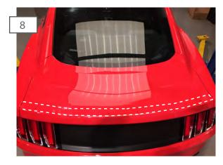
Prepare the decklid by cleaning it with the supplied alcohol pads. Allow time to dry.
