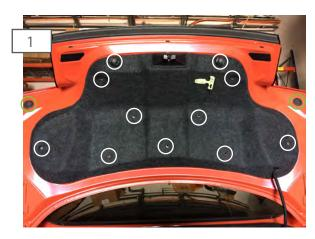
If equipped with a factory spoiler, remove the trunk lid trim panel. It is held on with (9) push pins and (2) rubber bumpers. With the panel removed loosen the bolts securing the spoiler. Remove the rubber covers (circled in green above) to gain access to the remaining spoiler bolts. The spoiler is also held on with tape carefully. Carefully remove the spoiler.
