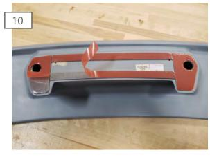
Peel back the tape backing from the center mount and apply adhesion promoter to the tape. Allow time to dry.
