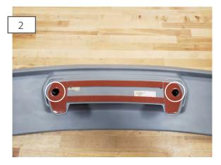
Install the center mount to the spoiler using the (2) hex head screws using a philips head screw driver.
