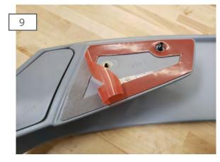
Peel back the tape backing from the side bracket mounts and apply adhesion promoter to the tape. Allow time to dry.
