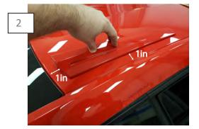
Test fit the roof splitter onto the roof. Measure 1" from the rear roof line forward, and 1" from the side roof line in. Mark the location of the roof splitter with painters tape. Do the same for the opposite side.
