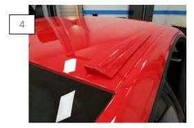
Align the splitter with the marks made in Step 2. Install the roof splitter to the roof. Apply firm even pressure to tapped surfaced to ensure proper adhesion. Do the same for the opposite side. Installation is now complete.
