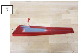
Peel back the 3m tape backing from the splitter, and apply the adhesion promoter to the tape. Allow time to dry.
