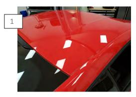
Clean the roof area with soap and water to remove any dirt or debris. Then using the supplied alcohol pads, further clean the surface to ensure best adhesion results.
