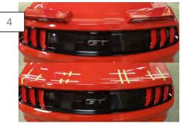
Test fit the spoiler to determine location by aligning all three pieces with the back edge of the decklid while making sure all three pieces are centered. Use the middle panel to determine the correct spacing between the two spoilers. Tape the template to the decklid where they lay. Carefully remove the spoilers from the templates. \*\*Note: This is the most important step so that the hole locations are drilled in the correct place.
