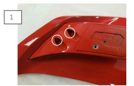
Install the side bracket to the spoiler using (2) M6x1.0x25mm Phillips head screws, and flat washers. The brackets are marked L or Left, and R for Right.
