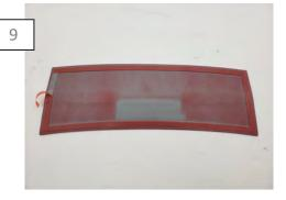
\*\*NOTE: Middle panel is optional to customers who did not have a factory spoiler. This panel will cover the factory middle spoiler hole locations for customer who did have a factory spoiler. Install the middle panel by removing the tape backing, and applying adhesion promoter to the tape. Allow time to dry. Insert the middle panel in-between the two spoilers. Apply firm even pressure to tapped surfaced to ensure proper adhesion.
