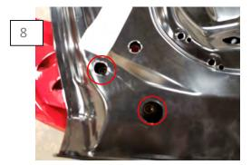
With a helper, start the (2) M6x1.0x20mm screws with washers on the outer spoiler mount, and (2) M6x1.0x15mm screws with washers in the inner spoiler mount to hold the spoiler in place. Apply firm even pressure to tapped surfaced to ensure proper adhesion. Do the same for the opposite side spoiler. \*\*Note: It's recommended to use a magnetic screw driver to prevent dropping hardware into the decklid.
