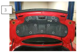
If equipped with a factory spoiler, remove the trunk lid trim panel. Remove the (9) push clips, and (2) rubber bumpers. With the panel removed, loosen the bolts securing the spoiler. Remove the rubber covers (circled in green above) to gain access to the remaining spoiler bolts. The spoiler is also held on with tape. Carefully remove the spoiler. \*\* Caution: Trunk lid is very thin and dents easily. \*\*Note: All remaining tape & residue needs to be removed prior to continuing to the next step.
