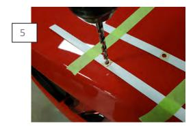
Using a drill & 1/4" drill bit, carefully drill the center of the template holes. Finish with a 7/32's drill bit on the back side. \*\*Note: Use touch up paint to any metal to prevent rusting.
