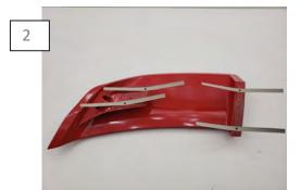
Remove the center adhesive backing of the supplied drill templates. Place the adhesive side on the spoiler, centering it over the bolt holes.
