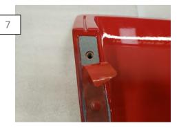
Peel back the tape backing from the mounting locations, and apply the adhesion promoter to the tape. Allow time to dry.
