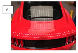
Prepare the decklid by cleaning it with the supplied alcohol pads. Allow time to dry.
