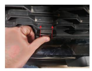
**Step 4** Gently apply firm pressure to seat the light into the grille to secure.
