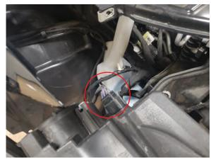
**Step 9**Once the headlight is unbolted from the vehicle unplug and remove the wiring harness from the light.
