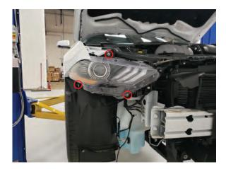
**Step 8**Remove the factory headlight from the vehicle using a 10 and 13mm socket.
