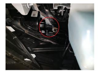
Step 6 With the splash shield removed, you can access the plugs for the turn signals and fog lights. Then remove bumper.
