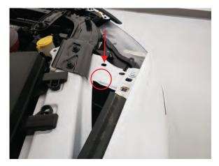
**Step 11**Using a Phillips or Allen key, use the attached adjustment screw to adjust the headlight to the factory specifications which can be found in the owners manual.
