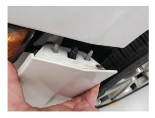
**Step 7**Once the bumper cover is ready to remove, using firm pressure pull the edge of the bumper down to pop it from the clip. Have a helper support one side so that you don't scratch the paint. Slowly remove the bumper and support it on a soft non-abrasive surface.
