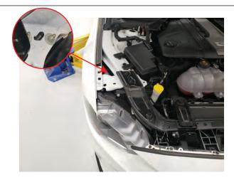
Step 5 From the top between the fender, locate and remove the (2) 10mm nuts then remove the bracket.
