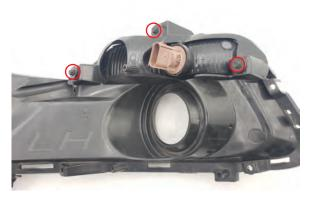
**Step 9** Remove the (3) 7mm screws securing the factory turn signal light to the foglight bezel. Remove the turn signal light.
