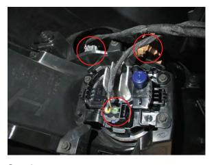
**Step 6** With the splash shield pulled back, you can access the plugs for the turn signals and fog lights. Then remove bumper.
