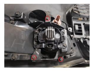
**Step 7** Remove the (3) 7mm screws securing the factory foglight to the foglight bezel. Remove the foglight.
