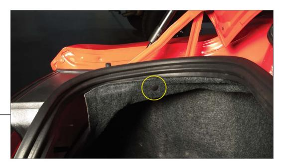
Using a panel removal tool, remove the (1) push clip securing the trunk trim in place.
