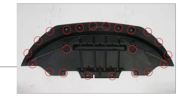
Support the front of the car so you can access the bumper splash shield. \*\*Note there are two versions of the splash shield. Both are attached to similar locations.
