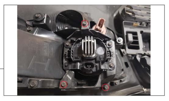
Remove the (3) 7mm screws securing the factory fog light to the fog light bezel. Remove the fog light.
