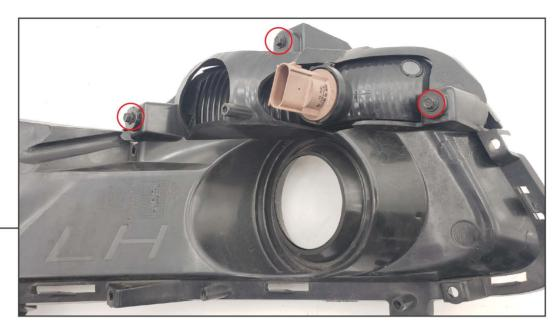
Remove the (3) 7mm screws securing the factory turn signal light to the fog light bezel. Remove the turn signal light. Install the replacement LED light using the factory hardware.
