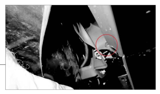
Fold back the fender liner so that you can access the one bolt that holds the bumper to the fender. Once removed, firmly pull the sides of the bumper away from the fender.
