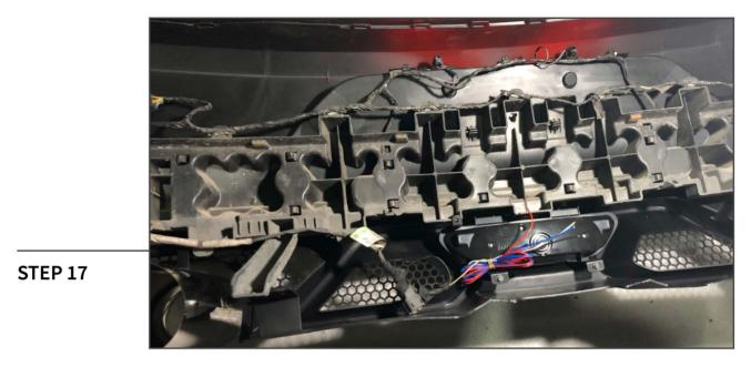
Then clip the bumper brace and wiring harness on to the bumper. Ensure electrical connector are plugged in.
