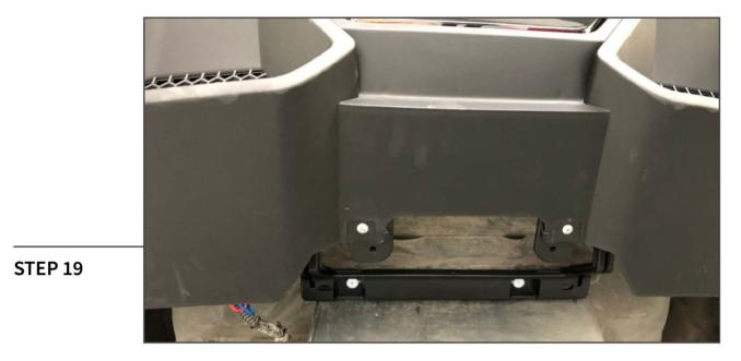
2015-2017 Vehicles: Install the rear valance/diffuser support between the rear valance/diffuser and the vehicle.
