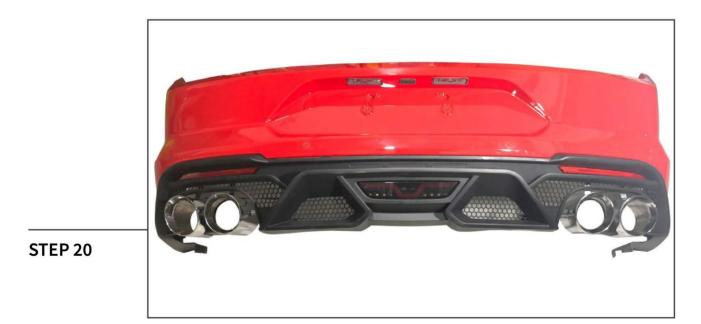
Clip the bumper on to the vehicle. Test the lights prior to reinstalling the bumper in reverse order. Ensure the electrical connection removed in Step 8 doesn't get pinched between the metal and the bumper otherwise the bumper will not fit correctly. Installation is now complete.
