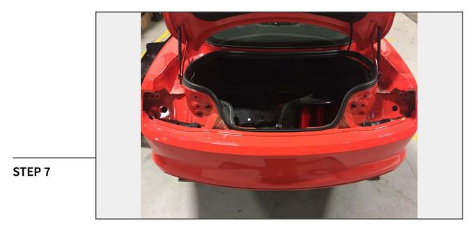
Firmly pull the bumper from the vehicle. The top edge of the bumper is held on with clips. Firm pressure will detach the bumper from the vehicle.
