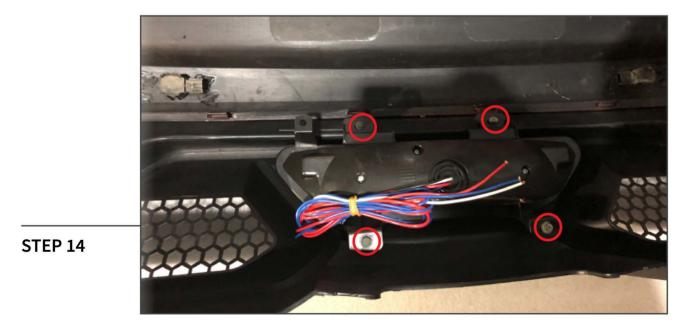
Transfer the reverse light from the factory bumper to the new bumper using the factory hardware.
