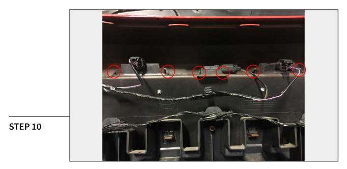
Unclip the license plate light housing and trunk button. Transfer them to the new bumper.
