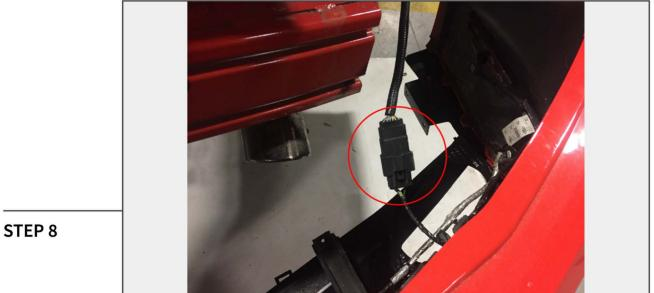
On the right hand side, locate and unplug the bumper wiring connection. Remove the bumper and place it on a soft surface.
