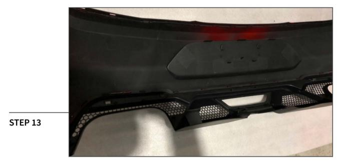
Install the rear valance/diffuser on to the bumper. Firmly press the valance/diffuser into the bumper. The parts will "click" together when properly install.
