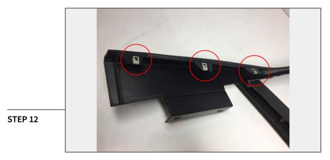
Transfer the screw clips from the factory bumper to the new rear valance/diffuser.
