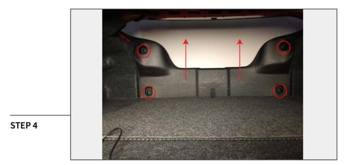
Remove the trunk trim panel by unscrewing the (4) cargo net fasteners. Pull the trim panel up and away from the vehicle.
