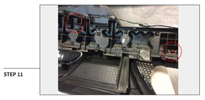
Unclip the rear bumper brace from the bumper. \*\*If equipped, unplug and removed the backup sensors to the new bumper.
