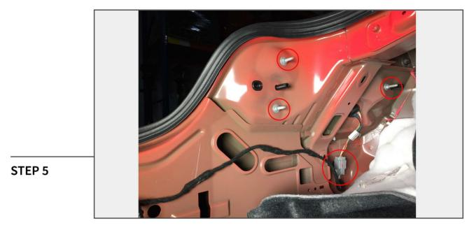
Fold back the inner trunk liners to access and remove the (3) nuts securing the tail lights to the vehicle. Unclip the electrical connections and remove the lights.
