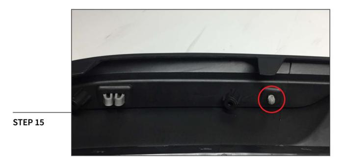
Using 10mm socket, remove the nut securing the rear bumper reflectors. Then transfer the reflectors to the new bumper. Reuse the factory nut.
