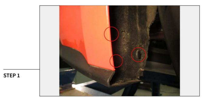
Raise and support the rear of the vehicle with a jack and support with jack stands. Remove the (3) plastic push clips that secure the fender liner to the bumper, repeat on both sides.
