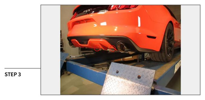
Remove the (2) 7mm screws securing the bumper to the bottom bumper bracket.
