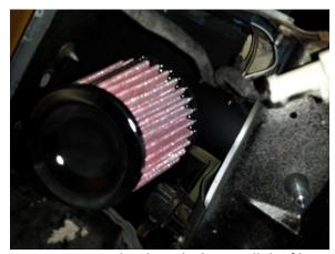
Step 9. From under the vehicle, install the filter onto the end of the tube.
