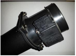
Step 5. Install the factory MAF sensor and housing to the lower part of the intake tube using the supplied gasket and hardware.
