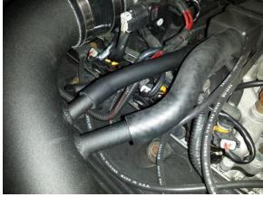
Step 8. Install the two vacuum lines to the upper intake tube assembly.
