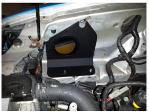
Step 2. Install the new shroud in the vehicle by sliding it into the factory mounting holes and securing it using the factory point at the top.
