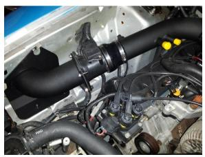
Step 6. Install the lower part of the intake tube onto the upper portion using the supplied coupler as show above and slide it into the shroud.
