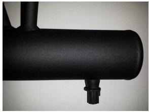
Step 3. Install the IAT sensor into the intake tube as shown.
