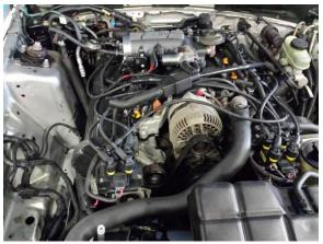
Step 1. Remove your factory intake, MAF sensor and IAT sensor from your vehicle. The IAT sensor and MAF sensor housing will need to be reused in the new intake assembly.
