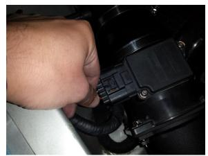
Step 7. Plug in the MAF sensor and IAT sensor using the factory wiring.
