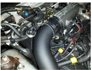
Step 4. Using the supplied coupler, fasten the intake tube to the throttle body. Leave it loose for adjustment.
