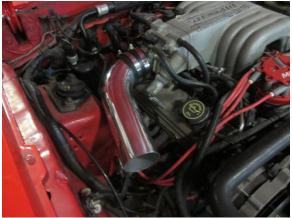
Step 2. Install the shallow tubing elbow onto the throttle body, leaving it loose for adjustments
