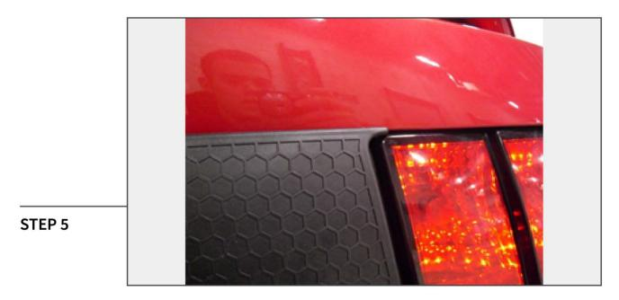
Peel backing from adhesive on outer panels and install on vehicle using the outer trunk lip and tail light as reference points. Once outer panels are properly located, press firmly down to fully seat the adhesive strips.
