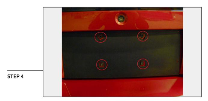
Peel backing from adhesive on center panel and install on vehicle. Use the license plate mounting tabs for reference when locating the center panel on the decklid. Once center panel is properly located, press firmly down to fully seat the adhesive strips.
