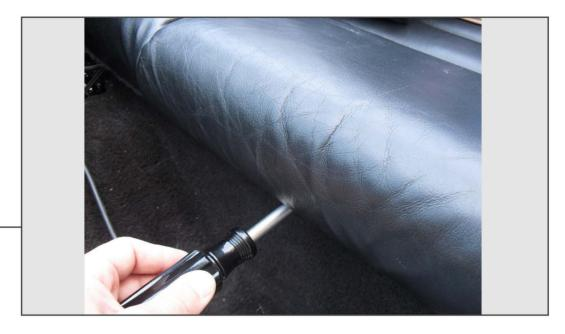
Use a flat-headed screwdriver to push in the retaining clips that hold the lower rear seat in place. Remove the seat from the vehicle.
