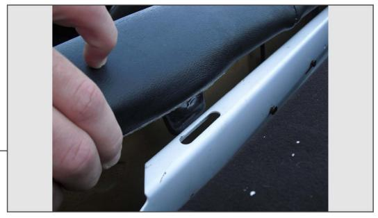
Once removed, pull up on the seat to release the upper clips holding the seat to the vehicle.
