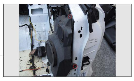
Remove the rear speakers from the vehicle by removing the two 7mm bolts that hold them to the body of the car.
