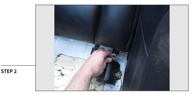
Remove the two 10mm bolts holding the upper rear seat in place.
