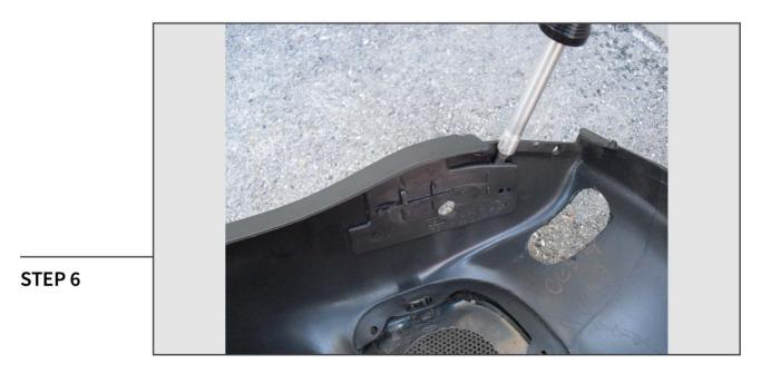
Once all holes are drilled, pry upper trim mounting clip from the panel as it is no longer needed.
