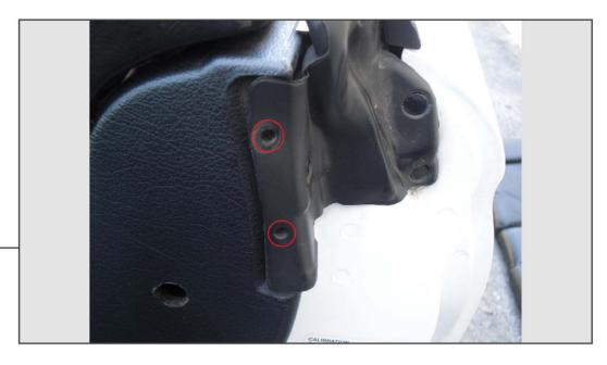
Remove the two pins holding the rubber seal to the trim panel, as well as the upper speaker grille using a flat-headed screwdriver to carefully pry the grille away. Use a torx head bit to remove the lower part of the seatbelt from the vehicle. Remove the rocker sill cover by carefully pulling upwards and removing from the vehicle. The interior panel should be free now and you will be able to remove it from the vehicle. Repeat Steps 3 &4 above to remove trim panel from opposite side.
