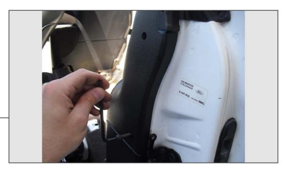
Once the brackets are properly secured to the body of the vehicle, re-install the inner quarter panel trim and out trim panel by reversing Steps 3 & 4 above. Carefully slide the styling bar into the holes you drilled in the interior panel trim. Push the bar down as far as it will go on both sides of the vehicle. Use the supplied hardware to
