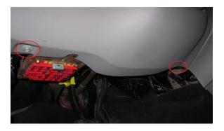
**Step 6:** Remove the metal column trim using an 8mm socket as well.
