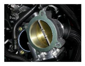
5. Using the supplied longer hardware, reinstall the throttle body, throttle body spacer assembly.
