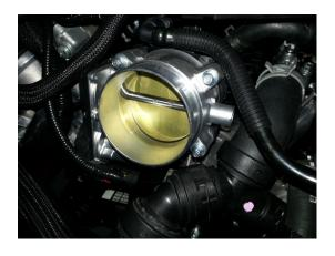
4. Place the supplied gasket between the throttle body and the spacer.
