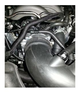
Using an 8mm socket, remove the 4 bolts holding the throttle body to the intake manifold
