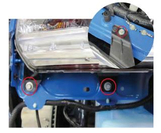
**Step 6** Remove the (3) 10mm bolts securing the headlight to the vehicle.
