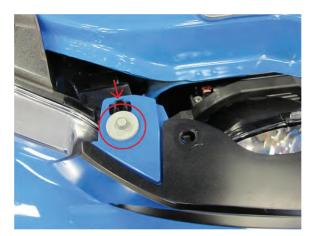
**Step 4** Remove the two 8mm bolts holding the top of the front bumper cover on and pull the cover over the black plastic tab shown in the photo below.
